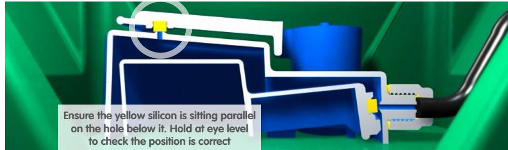
Ensure the yellow silicon is sitting parallel on the hole below it. Hold at eye level to check the position is correct
